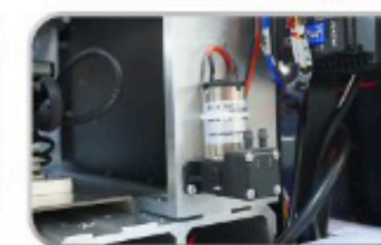
White ink stirring circulation system,Extend sprinkler life
